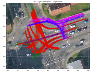
Figure 2: Real world picture of the intersection in Brunswick (Lines are representing detected trajectories red: vehicles, blue: bikes, pink: pedestrians, green: trucks)
