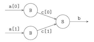
The assembly process server S is preceded by buffers. The server receives an item from each buffer B, before starting assembly. The received items are assembled into one new item, a list of its (sub-)items. The description of the assembly server is:
